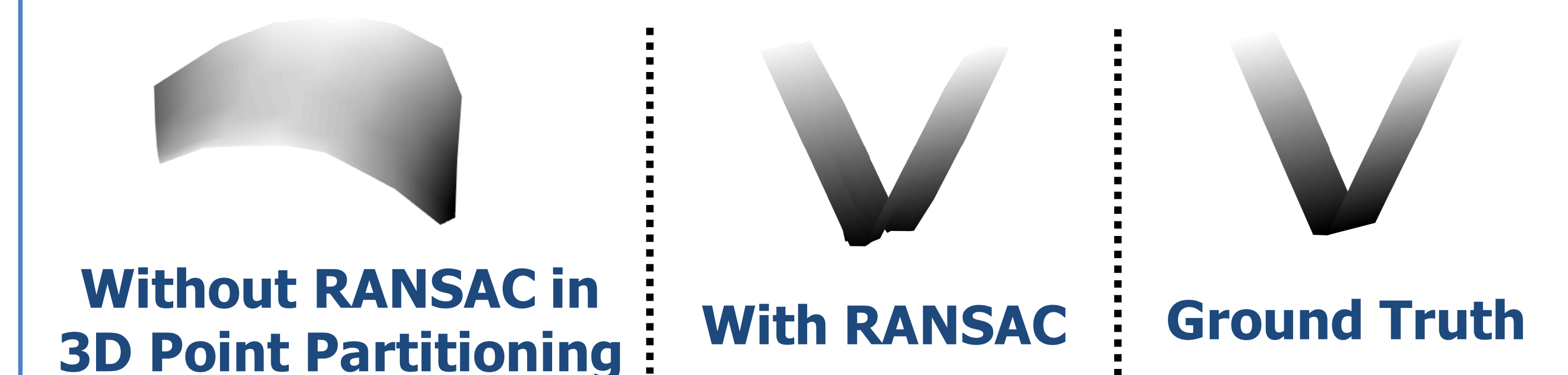
Fig. 2: Using RANSAC to partition points preserves the structure in the depth map of syn_crease
